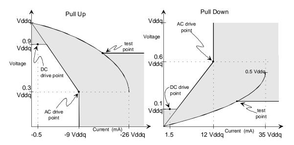
Equation A: Equation B:  $I_{Oh} = (54.0/Vddq)*(V_{out}-Vddq)*(V_{out}+0.4Vddq) \qquad I_{Ol} = (141/Vddq)*V_{out}*(Vddq-V_{out})$  for  $Vddq > V_{out} > 0.7 Vddq$  for  $Vddq > V_{out} > 0.7 Vddq$
