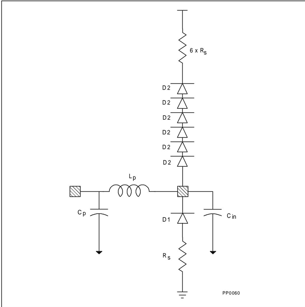
Figure 11. Input Buffer Model for Special Group
