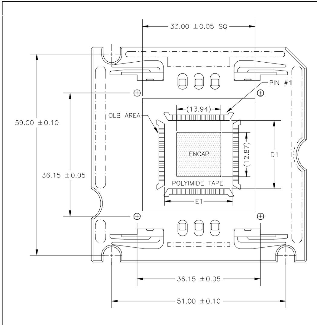
Figure 17. One TCP Site in Carrier (Top View of Die)
