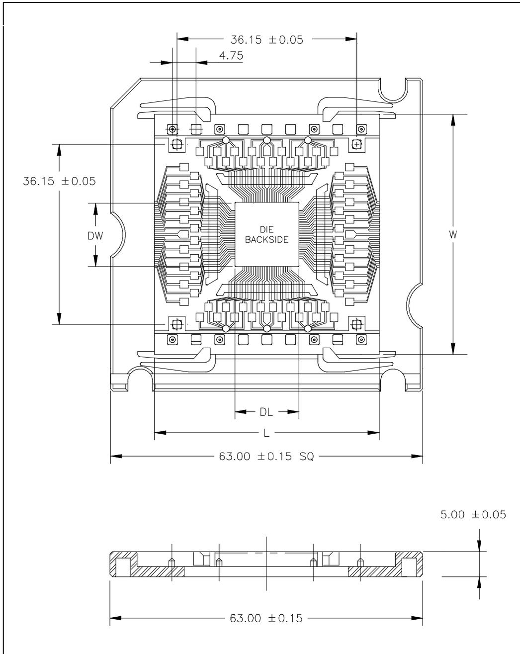
Figure 16. One TCP Site in Carrier (Bottom View of Die)
