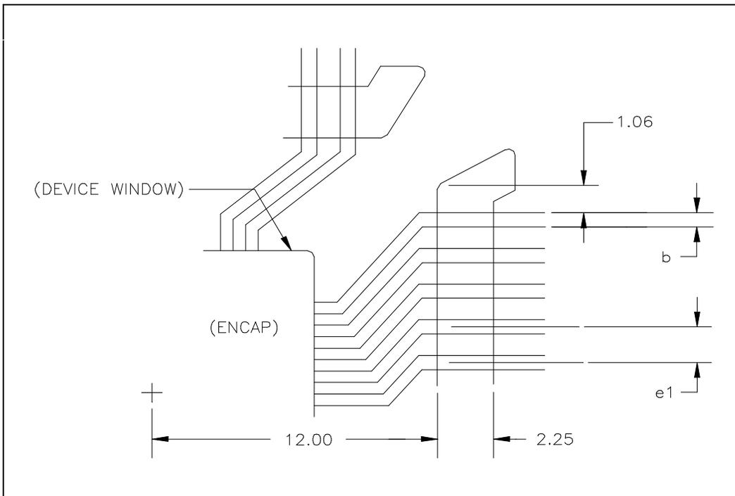
Figure 19. Outer Lead Bond (OLB) Window Detail
