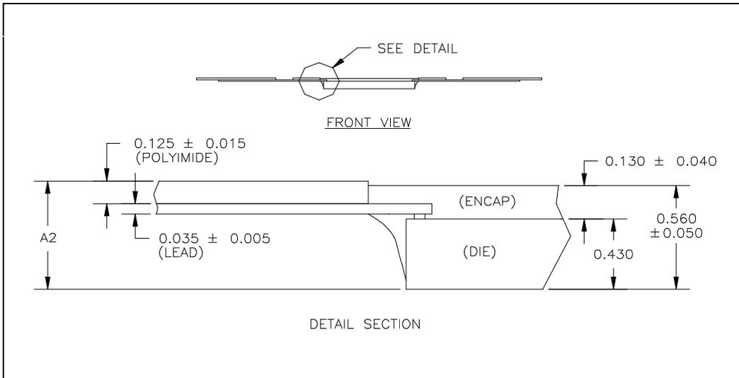
Figure 18. One TCP Site (Cross-Sectional Detail)
