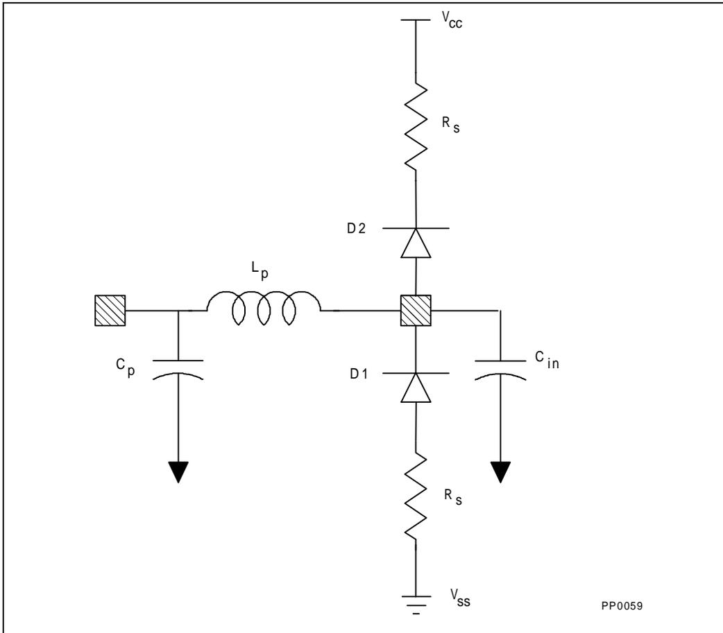
Figure 10. Input Buffer Model, Except Special Group
