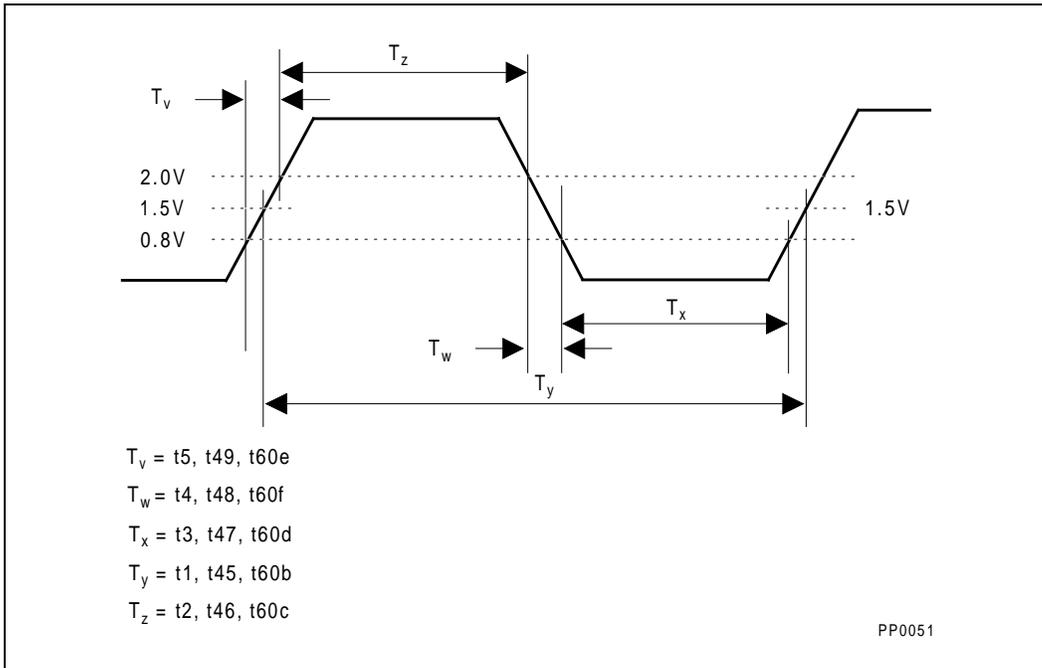
Figure 3. Clock Waveform
