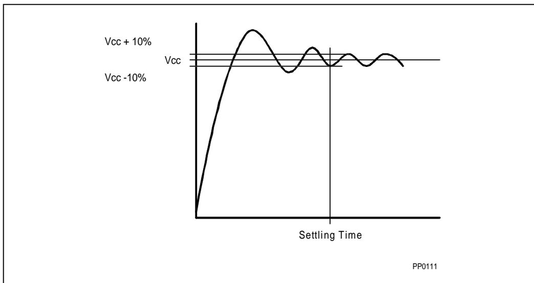
**Figure 14. Settling Time**
