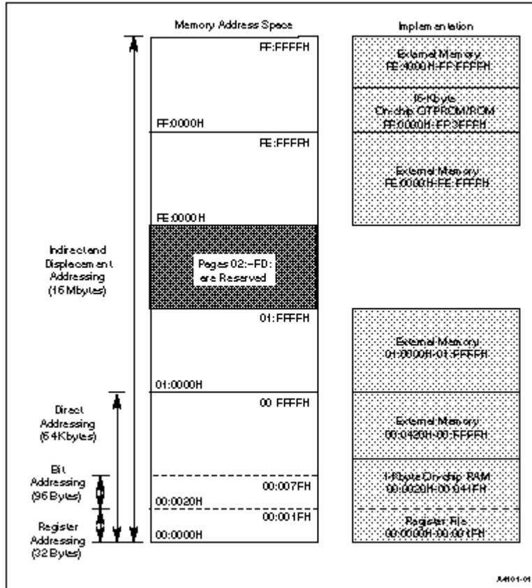
Figure 3. 8XC251SB Memory Mapping
