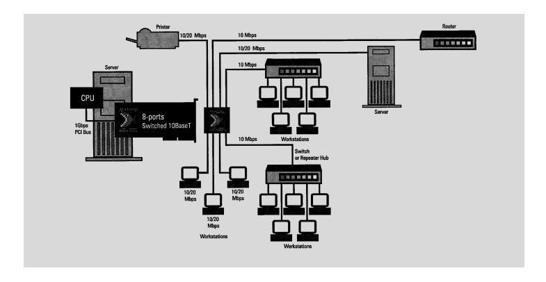
non-blocking switching architecture is based on a dedicated i960 RISC processor and an internal 1 Gbps PCI bus, providing wire speed switching on all LAN segments.
