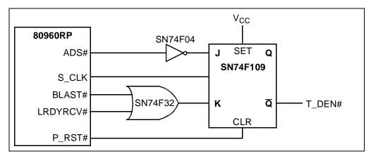
The circuit asserts T\_DEN# (Q#) at the start of the first data cycle when ADS# asserts and BLAST# and LRDYRCV# de-asserts. T\_DEN# deasserts at the end of the last data cycle when ADS# de-asserts and BLAST# and LRDYRCV# assert. During RESET, T\_DEN# de-asserts.
