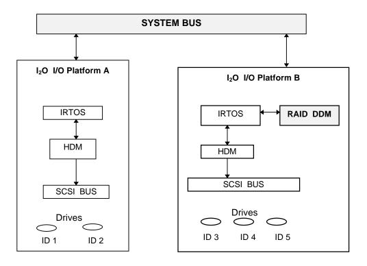
Through the I<sub>2</sub>O interface, the RAID module can control any and all of the five physical devices shown in the illustration and can reside on either Platform A or Platform B. The characteristics of either platform's SCSI bus and the system bus are hidden from the RAID module.
