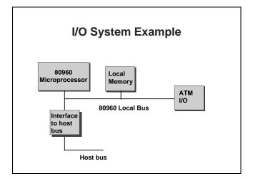
The diagram above shows a simplified example of how the 80960 would look in an ATM system or on the PCI-SDK board. I've generalized the ATM peripherals into one box labeled ATM I/O - this would contain a SAR (segmentation and reassembly) chip, physical layer devices, etc. On a PCI-SDK this would be the interchangeable I/O target module. There is also a box labeled "interface to host bus." On the PCI-SDK, this is the PLX 9060 PCI to 960 bridge chip.
