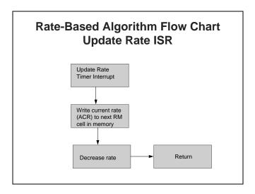
There are seven source / destination rate parameters that are used to calculate and specify data rates. These rates are initialized at call setup. The ACR is periodically recalculated by the source based on incoming RM cell information. The other six parameters are not changed for the duration of a call.
