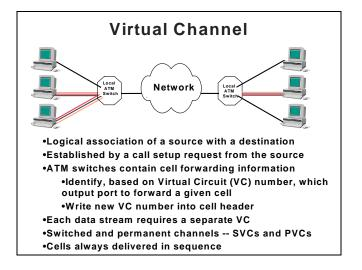
A virtual channel is the logical association between the source and destination. It's termed a virtual channel because unlike a circuit switched network, such as your telephone, where the physical connection is dedicated to your call, the virtual channel is a logical mapping from the source to the destination.
