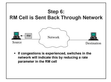
As the RM cell travels back through the network to the source, each switch must examine the ER value in the RM cell and determine if it can support that rate. If not, it must reduce the ER to the rate it can support. Step 7:
