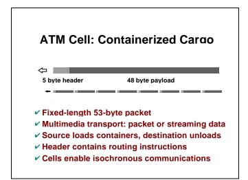
ATM is a cell switching technology. It relies on predefined paths, called virtual channels, to move cells through ATM switches across a network
