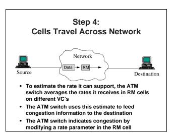
The network switches will mark the RM cell based on congestion encountered:
