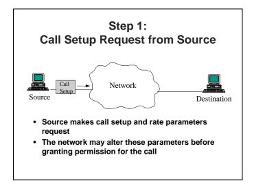
A connection from the source end station to the destination end station is initiated by a call setup request from the source. During the call setup, rate (and other) parameters will be negotiated with the network. After the network has granted permission for the call, rate parameters such as the peak cell rate and the minimum cell rate are initialized to the values that the network has agreed to support.
