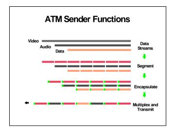
The sender's job is to get data to the destination. Let's take an example of three data streams that need to be transferred from point A to point B. Each stream of data has its own agreed upon data transmission rate. For example:
