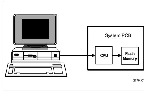
**Figure 1. The System CPU Controls In-System Writes to the Flash Memory Component**
