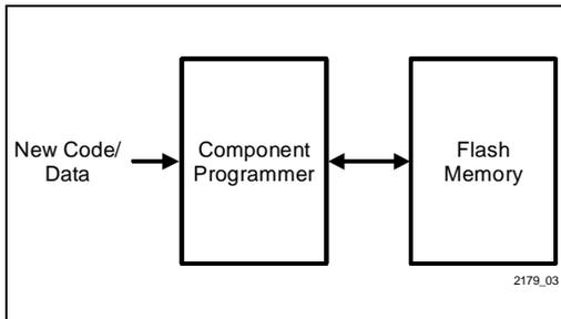
**Figure 3. The Component Programmer Controls Update of the Flash Memory**
