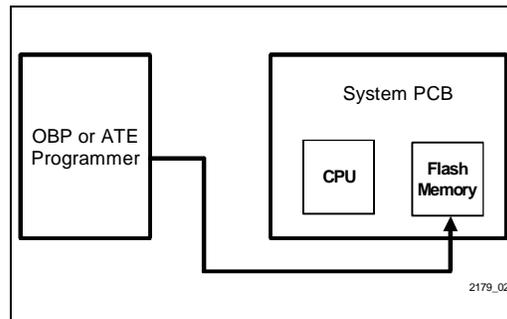
**Figure 2. The OBP Programmer or ATE Controls Flash Memory Update Operations**
