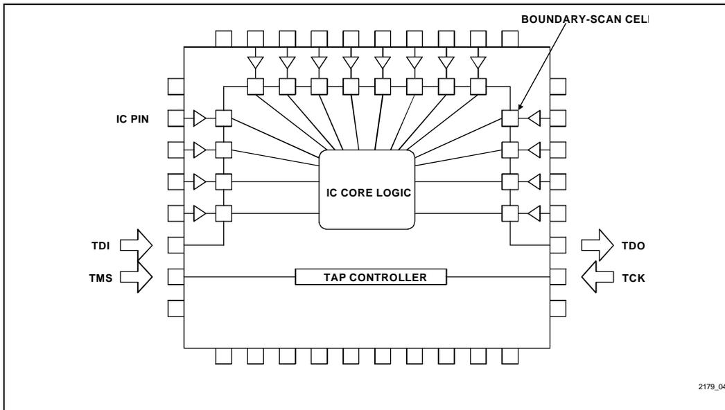
Figure 4. IC Containing JTAG Boundary-Scan Register
