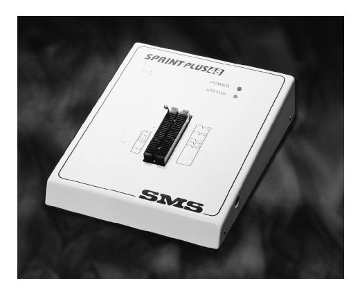
The PC interface is through the standard parallel port. With included software installed, the PLUS48 automatically interrogates LPT ports to determine where it is attached - then configures itself. Any LPT port, such as that on a notebook PC, can be used to control the PLUS48, giving you the freedom to take your support on the road.
