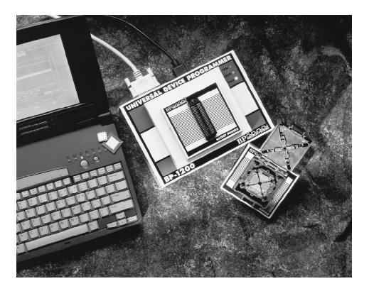
The BP-1200 design enables a trouble-free test vector operation. Short DUT trace lengths, excellent grounds at the socket, and fast rise and fall times allow programming and testing the fastest parts without trouble.
