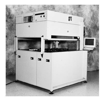
from 8 to 16 or even 24 programming stations. This results in constant high throughput, independent of the programming time of the devices. Each of the programming stations is controlled by its own PC to start programming immediately after inserting the device. That's why higher throughputs and best device support are achieved.
