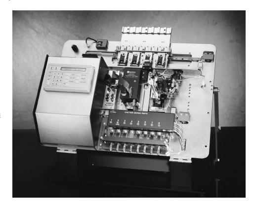
applications where traditional handling techniques are inappropriate or impractical. The PET 2 is perfect for characterization of devices and interfaces, programming and testing of surface mount devices.
