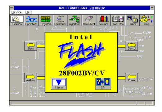
FLASHBuilder features a graphical representation of device functional blocks within the flash memory architecture as well as quick access to information about device operations, commands, algorithms and registers. For example, the command dialog box displays on a single screen the command set and corresponding hexadecimal values, bus-cycle counts for each command, and status register output indicating a successful operation.
