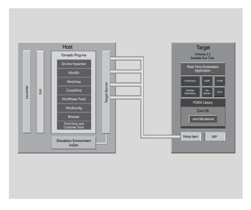
fast interrupt response. The microkernel design allows VxWorks to minimize system overhead and respond quickly to external events. To these features, VxWorks adds intertask communications and synchronization facilities, efficient memory management, multiprocessing support, a fast I/O system, IDE and SCSI support, and MS-DOS and RT-11-compatible file systems.
