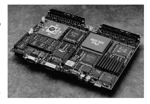
oriented programming and data security. With on-chip virtual-memory management, floating-point arithmetic, and multi-tasking capabilities, the i960 MC processor provides sustained instruction execution rates of 10 MIPs.
