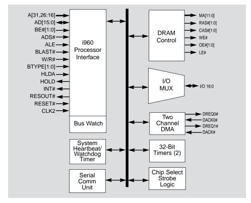
generation. In addition, the I/O lines may be used as simple I/O ports on a bit-by-bit basis. An on chip serial communications unit is also provided for connecting to either RS-232 or synchronous serial devices.
