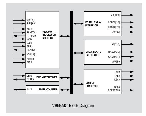
The V96BMC takes advantage of fast page mode DRAMs and row comparison logic to achieve static RAM performance using DRAMs.
