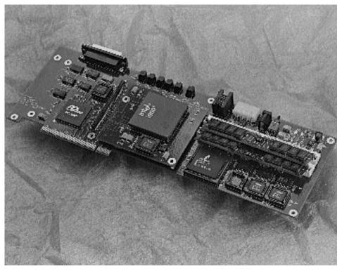
The PCI80960 supports Intel's GNU960 and other i960 processor software tools. It also supports pSOSystem and VxWorks real-time operating systems.
