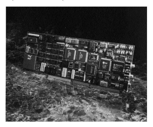
The heart of the compression/decompression engine consists of an ICC, an MEC, and an Intel i960® CA microprocessor. Compressed video bitstreams are transferred to and from the host PC under direct supervision of the i960 microprocessor. The i960 microprocessor is also responsible for video bitstream syntax handling and Huffman coding for the ICC chip.
