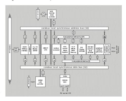
interfaces. This enables both the local bus and VMEbus to run at full speed, thereby enabling the board to achieve sustained VMEbus transfers of 54 Mbytes/sec.
