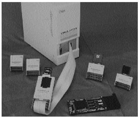
debugging or add optional debugging environments based on GDB960 or Microtec Research, Inc.'s XRAY Debugger. Other options include 4-8 MB emulation memory, a logic analyzer, workstation support, i960 processor upgrade kits (Sx, Kx, Jx, RP, Cx) and additional trace memory depth (to 32K cycles).
