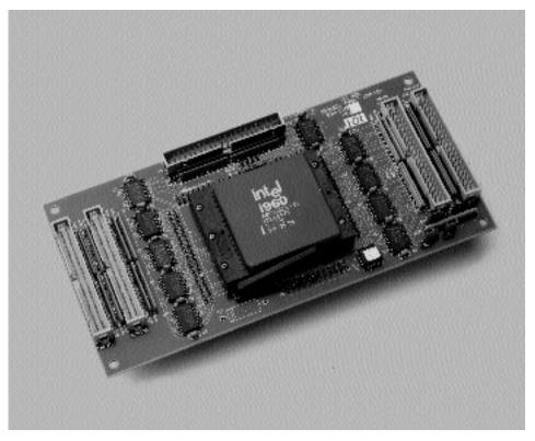
Another 100 MHz logic pod can be added to the system to monitor more processor signals. Four of these signals are user-jumperable, providing flexibility in hardware debug situations.
