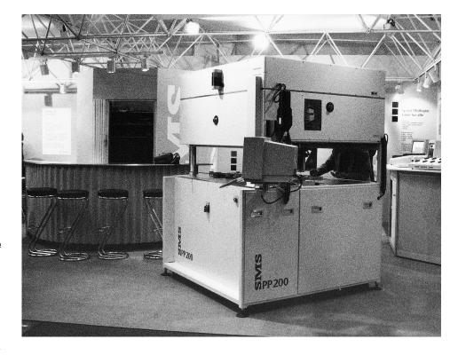
gantry and one pickup head with two vacuum suction cups can program, mark and sort up to 600 devices per hour.
