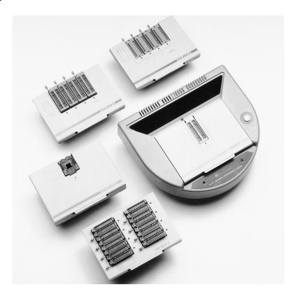
MICROCONTROLLERS SUPPORTED: 875x, 87C5x, 87C5xFx, 87C5xGx, 87C51Rx, 87C51Sx, 87L5x, 8xC251Sx,
