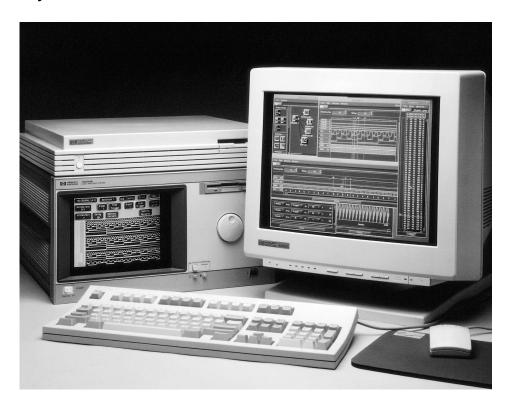
You can control and view data and perform post-processing analysis from the prototype analyzer's windows interface.
