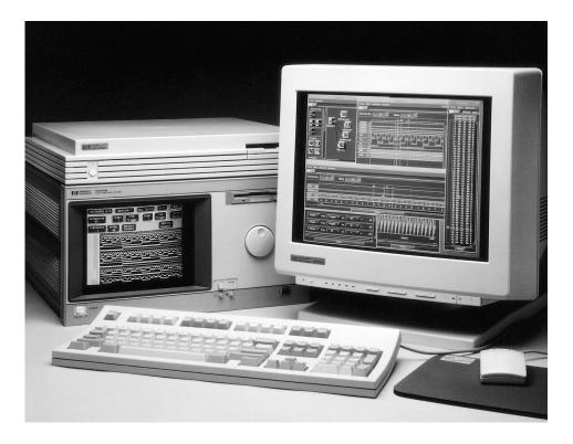
The HP 16500B logic analysis system consists of a mainframe that supports up to 5 independent measurement modules. An optional expansion frame supports an additional 5 modules.
