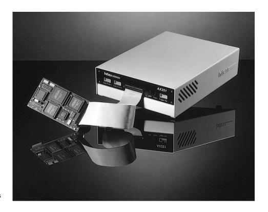
The hardware breakpoint system consists of separate 256K execution and 256K data access breakpoints. Execution breakpoints stop the emulation before executing the instruction where the breakpoint is set. Execution breakpoints can be set in ROM as well as writable memory.
