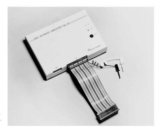
nal data memory spaces. There is also a watch window available to monitor C level variables in a user specified format (including support for local variables). Up to 10 breakpoints can be specified. Breakpoint conditions can include an address or address range in combination with the fetch, read, or write status and an external signal clip.
