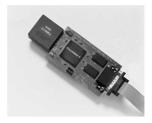
execution history clarity and can be fully qualified by any event in the Bus Event System. The timestamp uses 4 time bases -- 100 nsec to 1 msec -- that are independent of the target CLK; counter overflow is captured automatically to insure accurate long duration measurements. A special timestamp mode measures the MIN, MAX and MEAN interval time statistic for 4 independent events.
