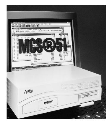
Microprocessor Development System. It provides real-time, non-intrusive, non-statistical Performance Analysis, Code Coverage and Report Generation, symbolic function-trace, time-stamping and timing analysis.
