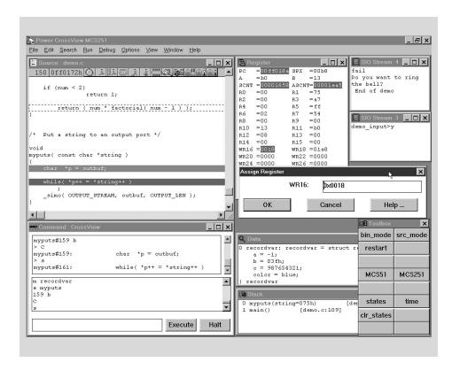
The simulator uses the same description file as the linker/locator when locating your application and therefore knows exactly where and how memory is mapped. It also has an alternate state counter to indicate which CPU execution mode (source or binary) is to be preferred for your application. All CrossView features, including C level trace and unlimited code/data breakpoints are available to you, so you can test code before target hardware is available.
