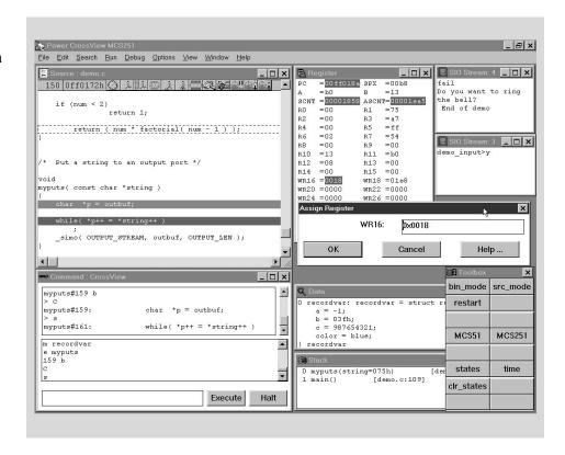
face, using a very efficient binary protocol. The resources used by the monitor program are kept to a minimum: it only uses 16 bytes of internal RAM, 3 Kbyte of code, one timer and the serial interrupt. MICROCONTROLLERS SUPPORTED: 8xC251Sx, 82930A
