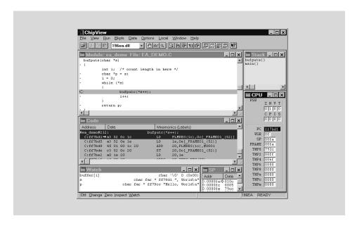
entire address space of the 24-bit family is simulated so that the Intel MCS 96 microcontroller program can be debugged on the simulator.
