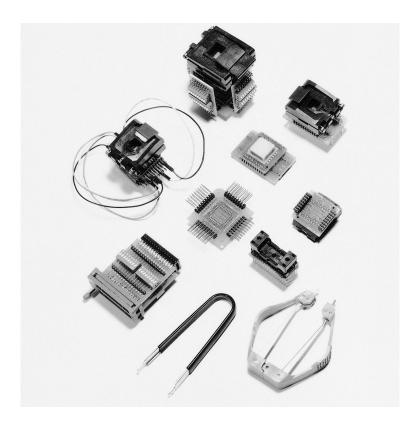
emulator connectors. Currently support is provided for 20 pin, 32 pin, and 44 pin targets. Please call us for our latest support for 68 and 84 pin packages.
