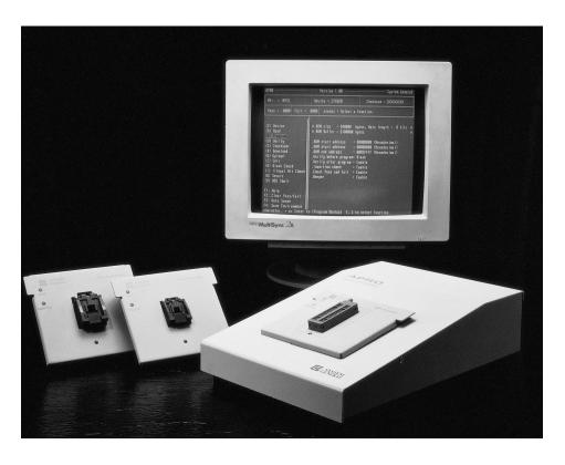
Default operation = Blank-check/ Program/Verify... Selectively disabled. MICROCONTROLLERS SUPPORTED: 875x, 87C5x, 87C51Fx
