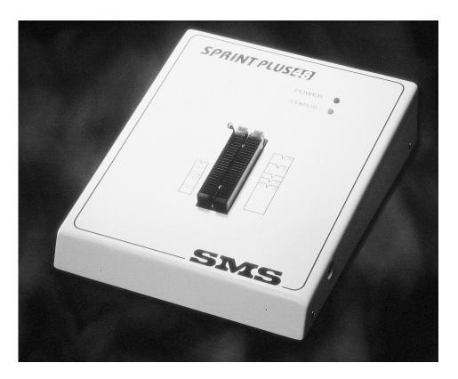
PC interface is through the standard parallel port. With included software installed, the PLUS48 automatically interrogates LPT ports to determine where it is attached - then configures itself. Any LPT port, such as that on a notebook PC, can be used to control the PLUS48 giving you the freedom to take your support on the road.
