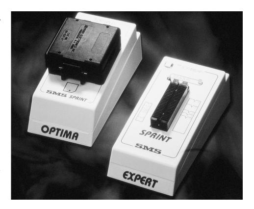
With the optional Power Pack, combine the OPTIMA with your favorite Notebook and you have a portable programmer that is ready to go anywhere. MICROCONTROLLERS SUPPORTED: 87C196Kx, 87C196Mx, 87C196Nx, 87C5x, 87L51Fx, 87C251Sx
